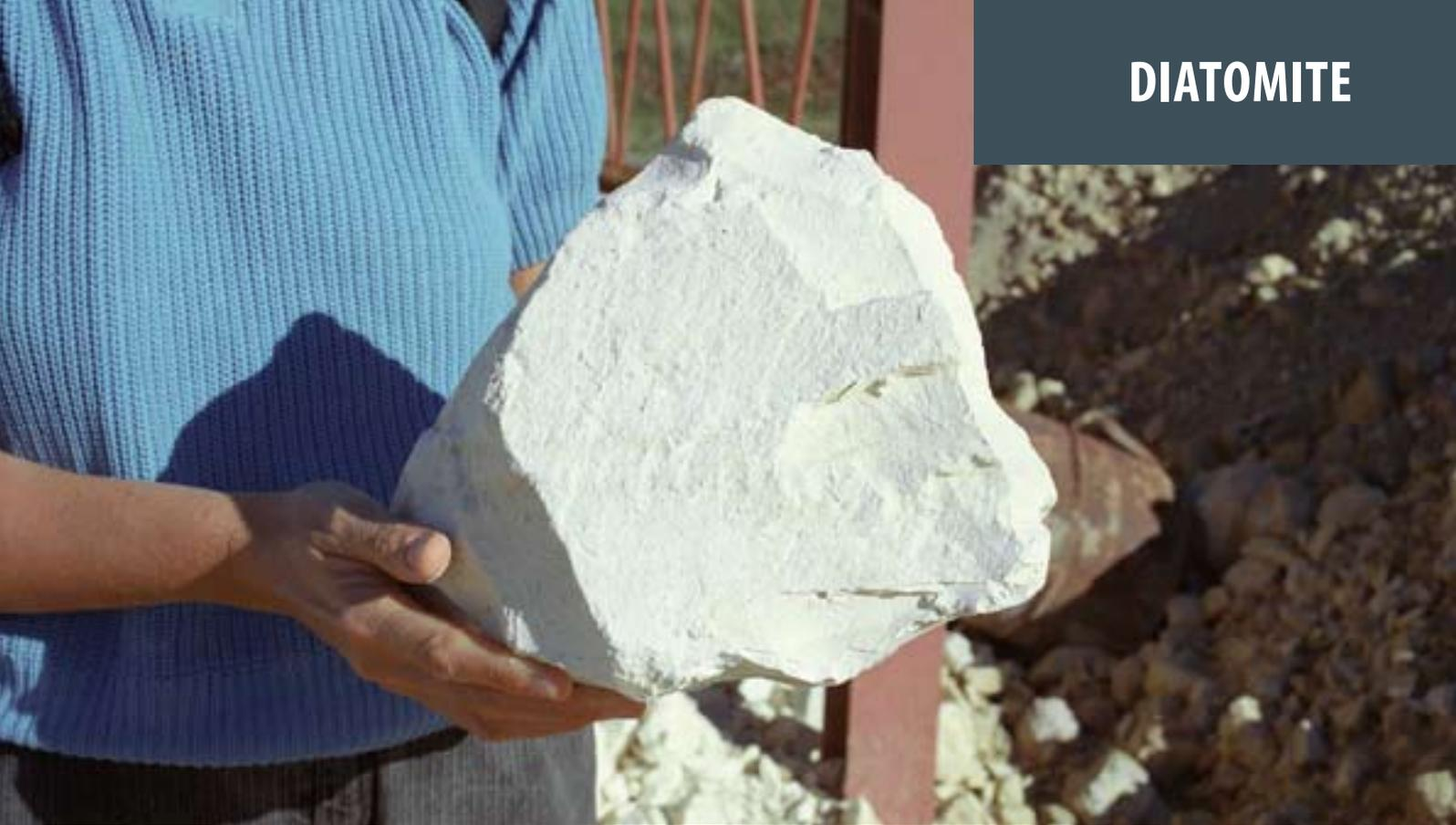
*Photograph 5. Diatomite from the Kyooma diatomite mine, Barraba. Diatomite is processed on-site and sold mainly for pet litter and for industrial and agricultural uses. The superior absorbency, chemical inertness and low density of diatomite allow its extensive use in industrial and domestic absorbents. (Photographer D. Barnes)*
